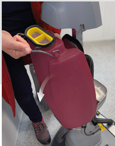
Recovery tank: remove
